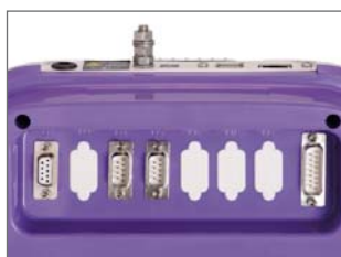
4 D-SUB connectors - IP40
