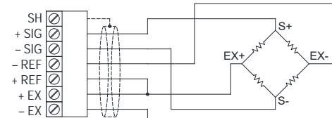
4 WIRES LOAD CELLS CONNECTION
