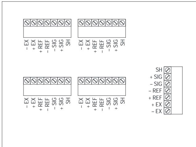
6 WIRES LOAD CELLS CONNECTION
